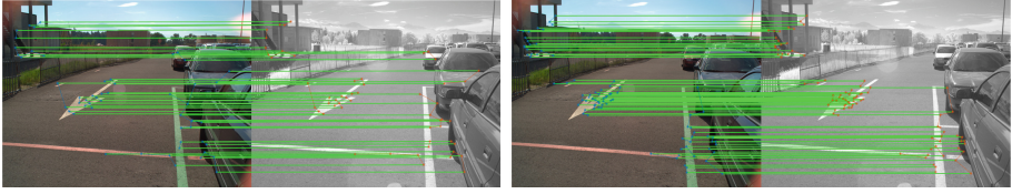
Fig. 4. Matching comparison between RGB/NIR image pair
