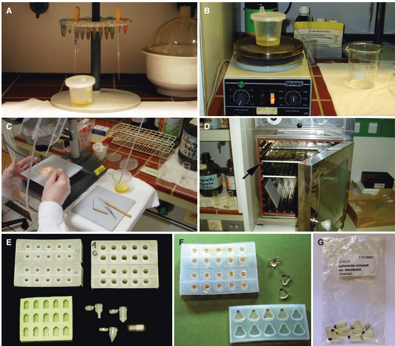
Fig. 12 Fixation and embedding day 2–4. A. Infiltration starts by repeatedly adding few drops of embedding media. B. Embedding solution (Agar low-viscosity resin) mixed using a magnetic stirrer. C. Final embedding into adequate embedding forms under binocular microscope. D. Polymerization at 70 °C in a thermostat oven (arrow). E. Examples of various embedding forms. F. Polymerized samples. G. Specimen blocks stored in small plastic bags
