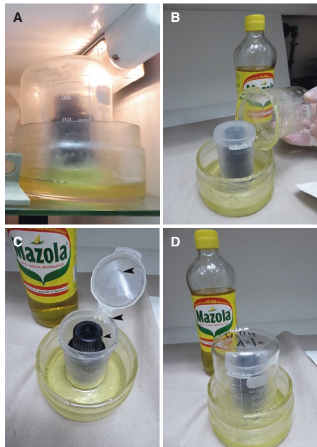
Fig. 28 Osmium storage. A. Osmium solution stored at 6 °C (fridge placed in a fume hood). B-D. Osmium solution in a sealed bottle and stored in a plastic container, plastic container placed in glass vessel containing oil. C. Arrowheads showing osmium contamination from volatiles. D. Second glass vessel placed over the osmium containers, osmium vapor is bound to the oil and cannot escape into the atmosphere
