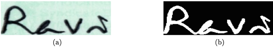
Fig. 3. K -means image binarization: (a) Color input image; (b) Binarized output image.
