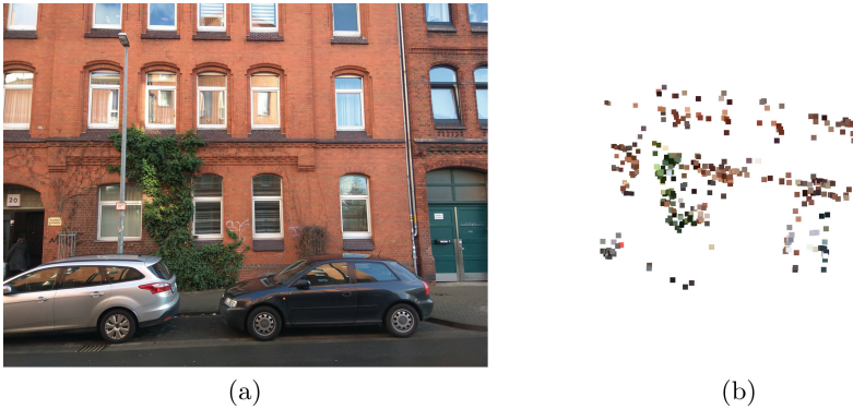
Fig. 7. A reference image and the corresponding sample sparse 3D reconstruction using the feature points from the refined set.
