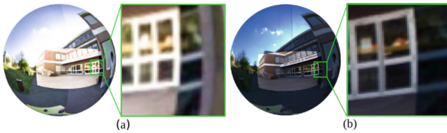
Fig. 7. (a) The image from fisheye and ZED cameras are fused together. (b) The fusion result after applying the projective distortion on the ZED image. Focusing to the border between ZED and unit sphere, the ZED image is perfectly over-lapped on the unit sphere.
