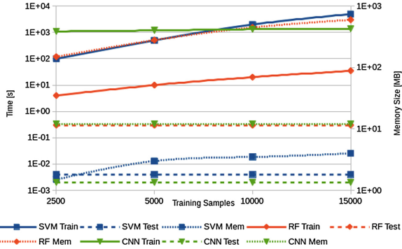
Fig. 4. Computational and memory footprint performance: training times—solid line, testing times—dashed line, and memory footprint—dotted line of the classifiers, versus the number of training samples
