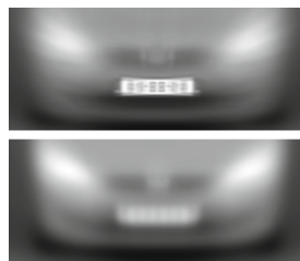
Fig. 6. Average automatically annotated detection box (top) and average detected result (bottom).
