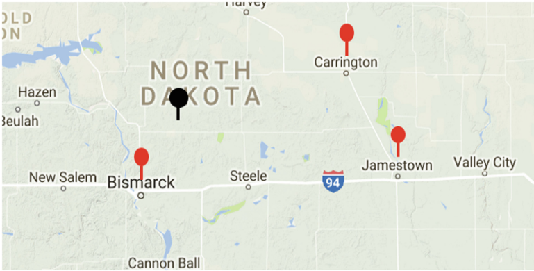
Fig. 1. An illustration of model results given a collective query of three cities (in red); the result (the town of Regan; name not shown on map) returned by the embedding model is the black pin. The embeddings reflect spatial proximity and can be used as feature vectors for the corresponding location entities in a machine learning pipeline. (Color figure online)
