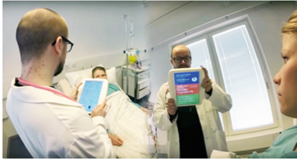
Fig. 1. The dual-sided tablet used in a hospital context. The front display shows electronic health record information, whilst the rear display provides the patient with visual information to support the consultation process.
