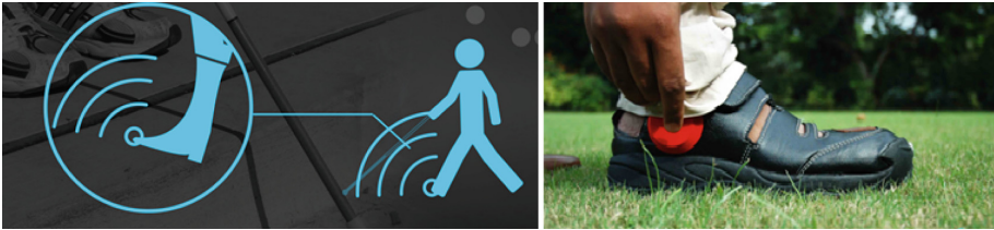
Fig. 1. Depicts ultrasound sensor that detects the obstacles (left). Depicts design of the Smart Shoes prototype (right).
