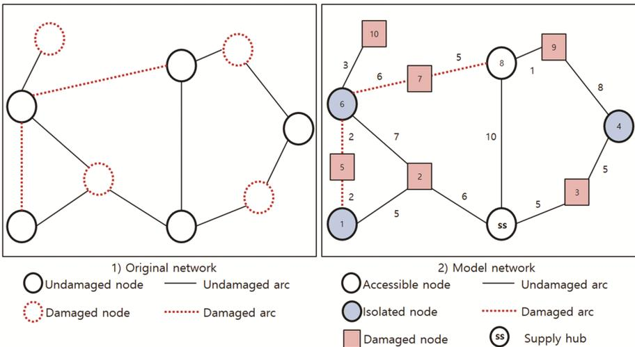
**Fig. 2.** Example of a damaged road network.
