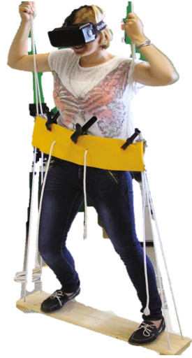
Fig. 1. Intermediate prototype from the iterative design process for a range of suspended setups for locomotion in VR.
