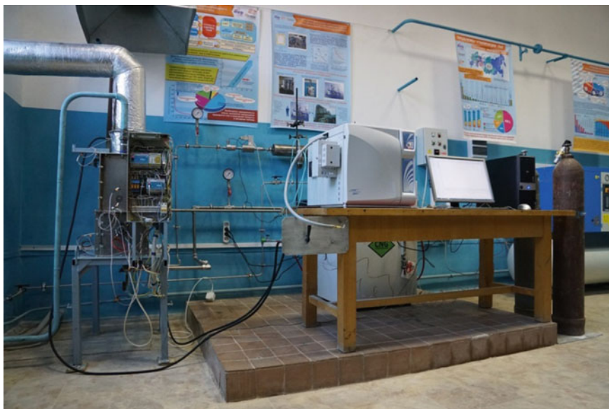
Fig. 2 Pilot installation for matrix conversion of natural gas at atmospheric pressure. Input natural gas capacity up to 20 \text{ m}^3/\text{h}
