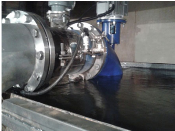
Fig. 5 Micro-hydraulic power plant mockup model on NRU “MPEI” experimental bench
