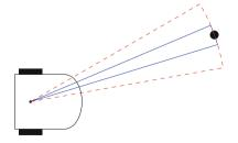
Fig. 2.3 Beam width of laser light (solid) and non-coherent light (dashed)
