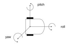
Fig. 2.11 Three-axis accelerometer
