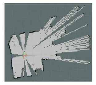
Fig. 2.9 A map of the environment obtained by a laser scanner
