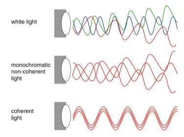
Fig. 2.4 White, monochromatic and coherent light
