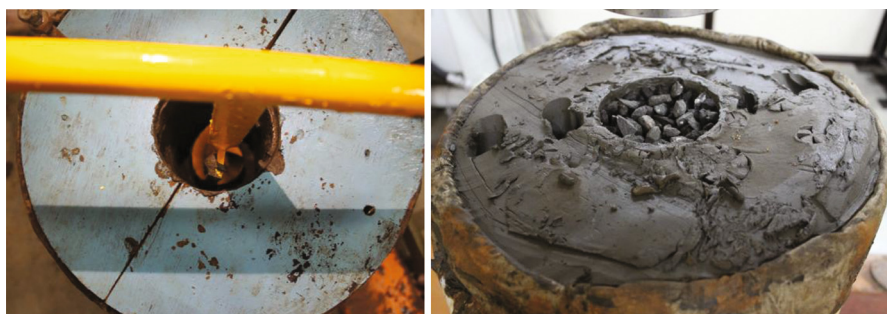
Fig. 4. Hole formed by auger and hole filled up with aggregates
