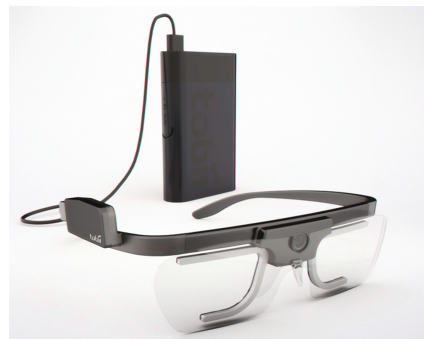
Fig. 2. Tobii Pro Glasses 2 [12]. A wearable gaze tracker that tracks a respondents eye movements using IR cameras, while also recording the environment with a front facing video camera.
