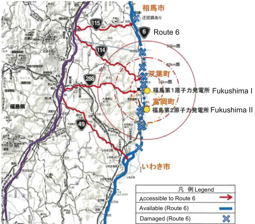
Fig. 1 Location of damage along Route 6. http://www.thr.mlit.go.jp/road/jisinkannrenjouhou_110311/dourohisaijoukyou.pdf
