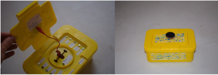
Fig. 7. The sound metaphor box , designed to teach the notion of size to young visually impaired children with associated disorders. It was made of a plastic box and small metallic screws (interactive zones). The Touchboard is hidden in the box.
