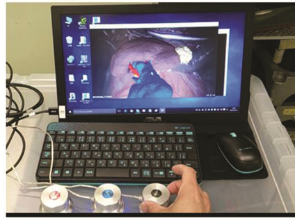
(b) Navigation system controller
