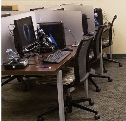
Fig. 1. Laboratory set up showing Gazepoint GP3 beneath a 17 inch monitor
