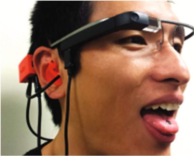
Fig. 5. Tongue magnetometer and Outer Ear Interface [28].
