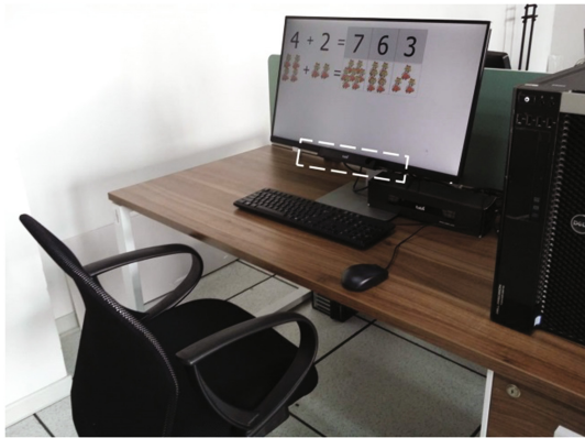
Fig. 10. The study environment where the dash-line highlighted Tobii X2-60 eye-tracker was mounted below the monitor
