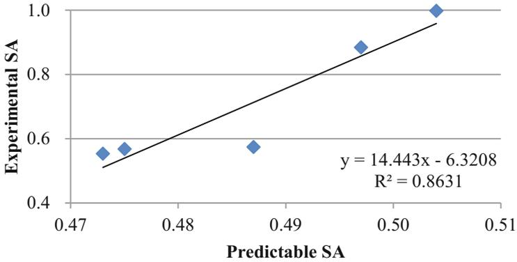
**Fig. 6.** Regression analysis of SA during take-off and climbing phase
