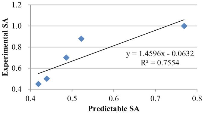
Fig. 8. Regression analysis of modified SA during cruising flight phase
