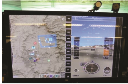
Fig. 12. Multi-touch multi-function Display (MFD) in the simulator cockpit.
