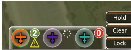
Fig. 6. UAV Dock. Left UAV has two tasks and warnings, center UAV is planning, and right UAV is offline. (Color figure online)
