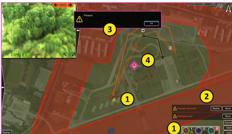
Fig. 7. Three levels of warning information: Symbols in dock and next to UAV (1), detailed description (2) and info dialog (3) with flashing object indicator (4).
