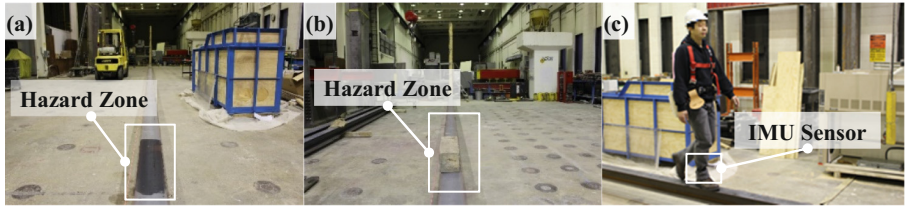
Fig. 1. Laboratory experiment environment. (a) Slippery surface, (b) obstacle, (c) subject participating in the experiment.
