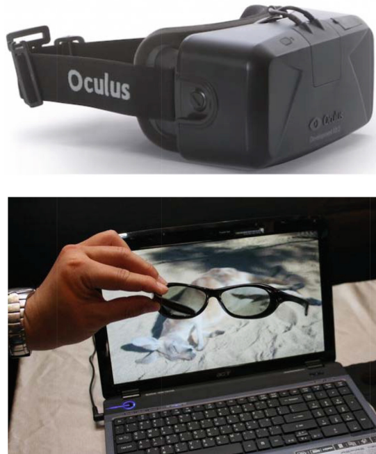
Fig. 1. Oculus Rift DK2 (above), and Acer Aspire 5738DG laptop with stereoscopic display (below)
