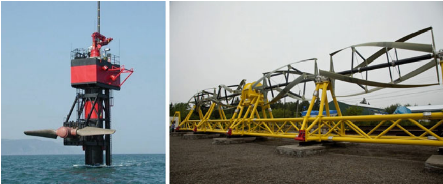
Fig. 3.6 Left Example of a tidal stream generator that converts the kinetic energy from marine currents (e.g. Gulf stream or tidal currents) into electricity. The technical concept is similar to that of a wind power station, but due to the high density of water compared to air, also the energy density is higher and the “propeller” can be much smaller. In the photo, the rotor is moved above sea level for maintenance. A “fence” of these current turbines can convert tidal power at large scale using existing technology. Right A chain of horizontal helical turbines is another option for hydropower generation [23]
