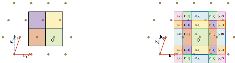
Fig. 1. Babai’s partition and the natural partition in dimension two: different cells are coloured differently. (Color figure online)
