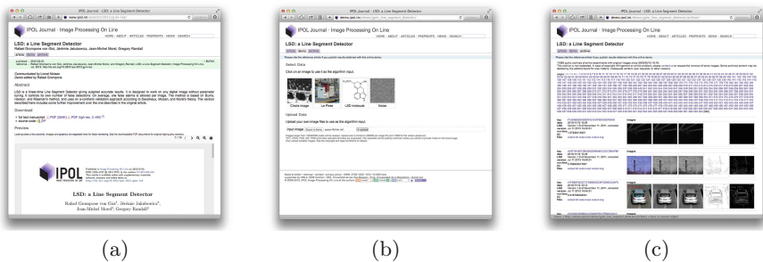
Fig. 1. The current form of an IPOL article with its three tabs: (a) article with manuscript, online viewer, and link to source code, (b) demonstration system, and (c) archived experiments.
