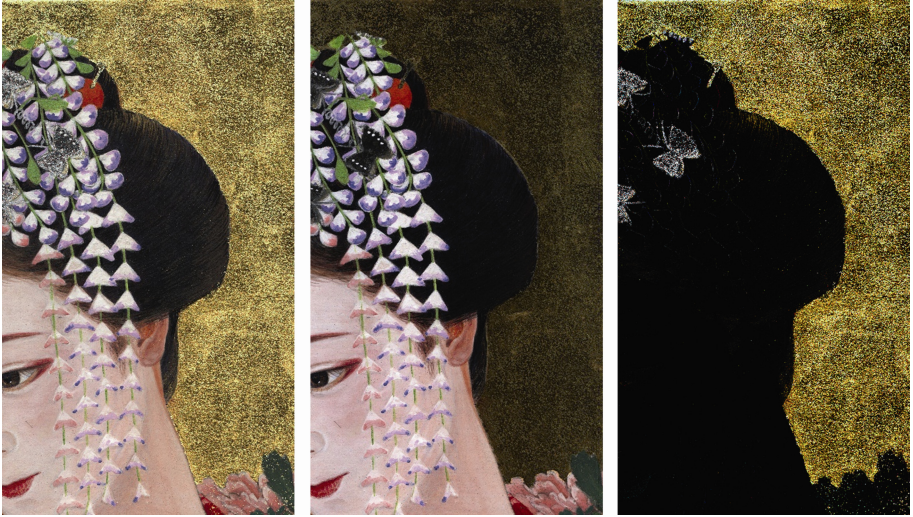
Fig. 13. Polarized light showing separation of diffused and specular reflection (painting 1). The image on left is the total reflection image, center is the diffuse light, and right is the specular image.
