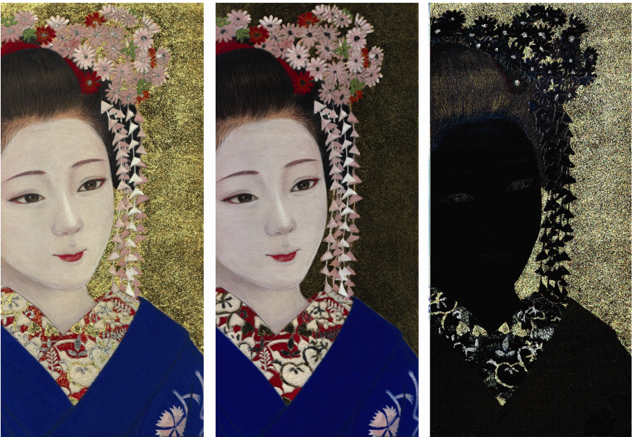
Fig. 14. Polarized light showing separation of diffused and specular reflection (painting 2). The image on left is the total reflection image, center is the diffuse light, and right is the specular image.
