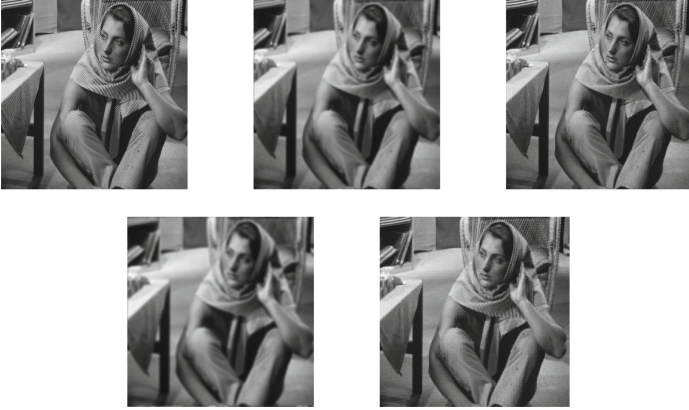
Fig. 1. Top line: exact image (left), Gaussian blurred image (middle) and MNP reconstruction (right). Bottom line: out-of-focus blurred image (left) and MNP reconstruction (right). The noise level is NL = 7.5 \cdot 10^{-3} .
