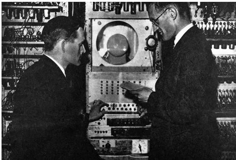
Fig. 8.1 Baby, the first electronic stored-program computer. Baby came to life in June 1948. The proud parents: Tom Kilburn is on the left, Freddie Williams on the right (Courtesy of the University of Manchester School of Computer Science)
