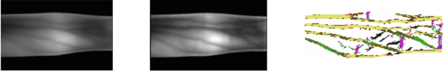
Fig. 2. The finger vein image used as running example (left), its enhancement (center), and the final segmentation (right).
