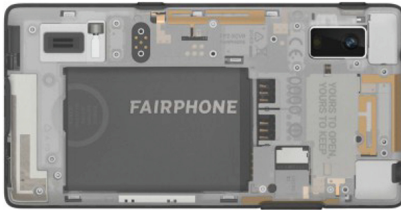
Fig. 3. Transparent back cover of the Fairphone 2
