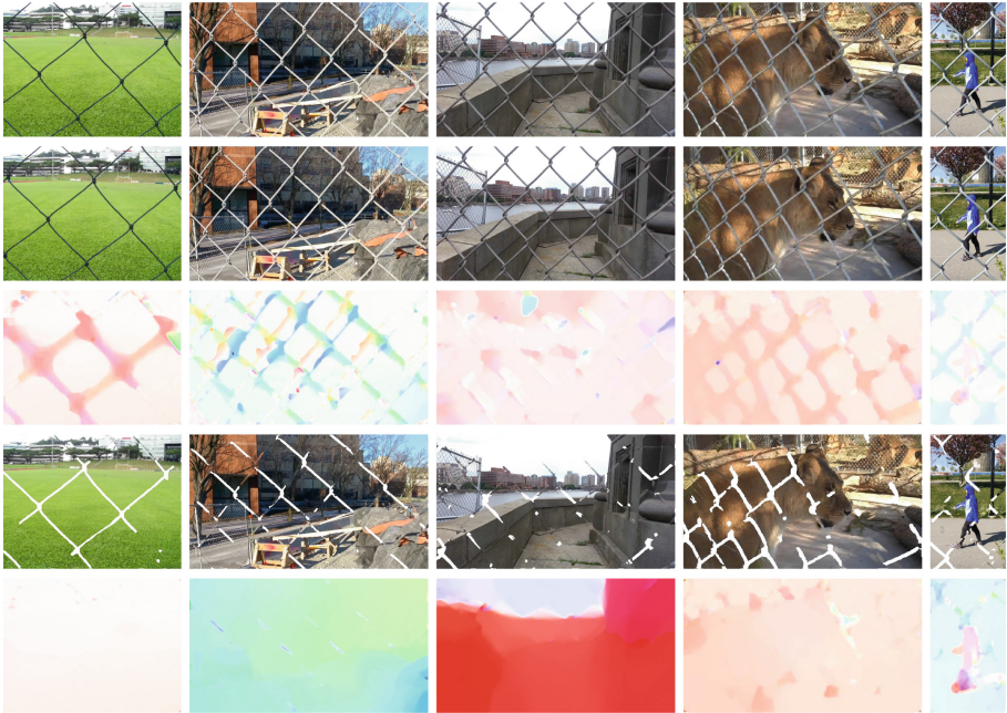
Fig. 6. First and second row: frames taken from videos reported in [6, 9, 10]. Third row: optical flow computed between the first and second row images using [24]. Fourth row: de-fenced images obtained using the estimated flow shown in the third row. Fifth row: occlusion-aware optical flow obtained using the proposed algorithm.
