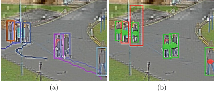
Fig. 4. Example of newborn particles generated at frame 43 (crop) in PETS09-S2L1. (a) Color-coded target identities; (b) existing particles (green dots) and newborn particles (red dots). The newborn particles initialize a new trajectory from an un-associated strong detection. (Color figure online)
