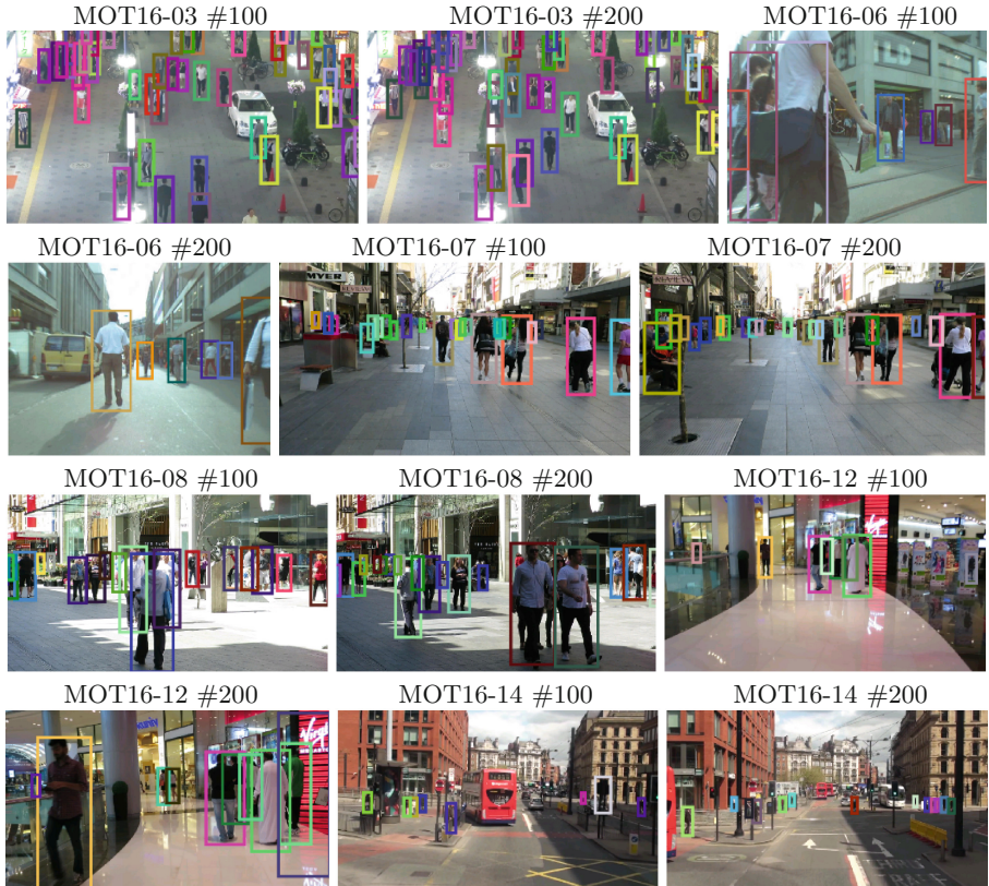
Fig. 5. MCMOT tracking results on the test sequences in the MOT Benchmark 2016. Each frame is sampled every 100 frames (these are not curated). The color of the boxes represents the identity of the targets. The figure is best shown in color. (Color figure online)
