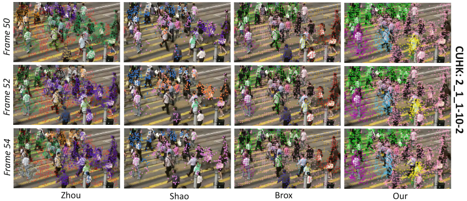
Fig. 1. Segmented motion patterns (or groups segregation) as the crowd evolves in time. The color of point represents the assignment to a group. While groupings are temporally consistent over a set of frames for Brox [2] and Our method. Zhou [3] and Shao [4] fail to maintain consistent groupings between frames. (Color figure online)
