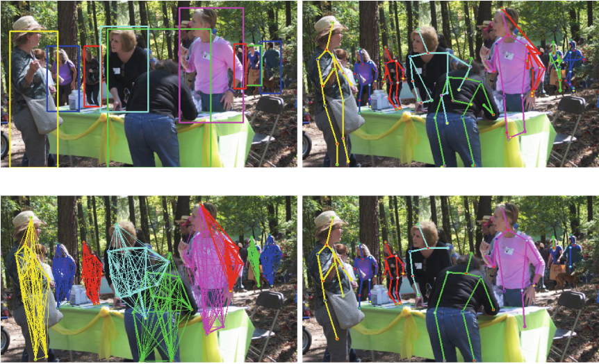
Fig. 2. Overview of the proposed method. We detect persons in an image using a person detector (a). A set of joint candidates is generated for each detected person (b). The candidates build a fully connected graph (c) and the final pose estimates are obtained by integer linear programming (d). (best viewed in color) (Color figure online)
