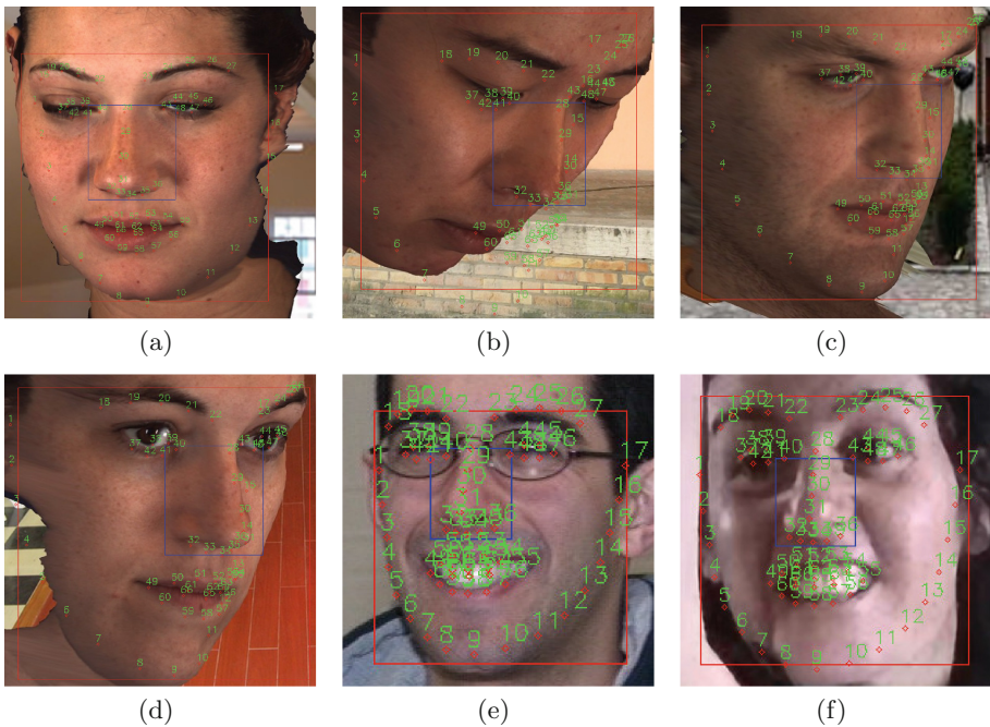
Fig. 3. Example results of the model fitting stage, showing the face bounding-box in red, the detected nose region in blue and the estimated position of the landmarks in green. (a) Near frontal good fit; (b) Bad fit caused by bad head pitch estimation; (c) and (d) Half-profile good fit; (e) Good fit in an image sourced from the MultiPIE dataset; (f) Modest fit in one of the most challenging images in the dataset (Color figure online)
