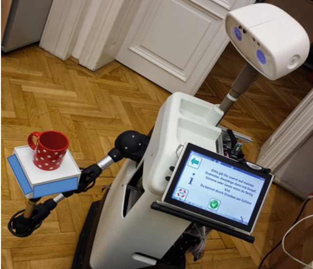
Fig. 1. The robot used for learning object models and then using the models for object detection. The robot is shown during the acquisition of the model of an object of interest. It uses an active robot head to direct an RGB-D camera towards the object. The object is placed on a turntable including natural script on its side walls (masked for reasons of anonymity). The user initiates the robot learning procedure and then the robot guides the user through the necessary modelling steps. The processing steps are executed autonomously.
