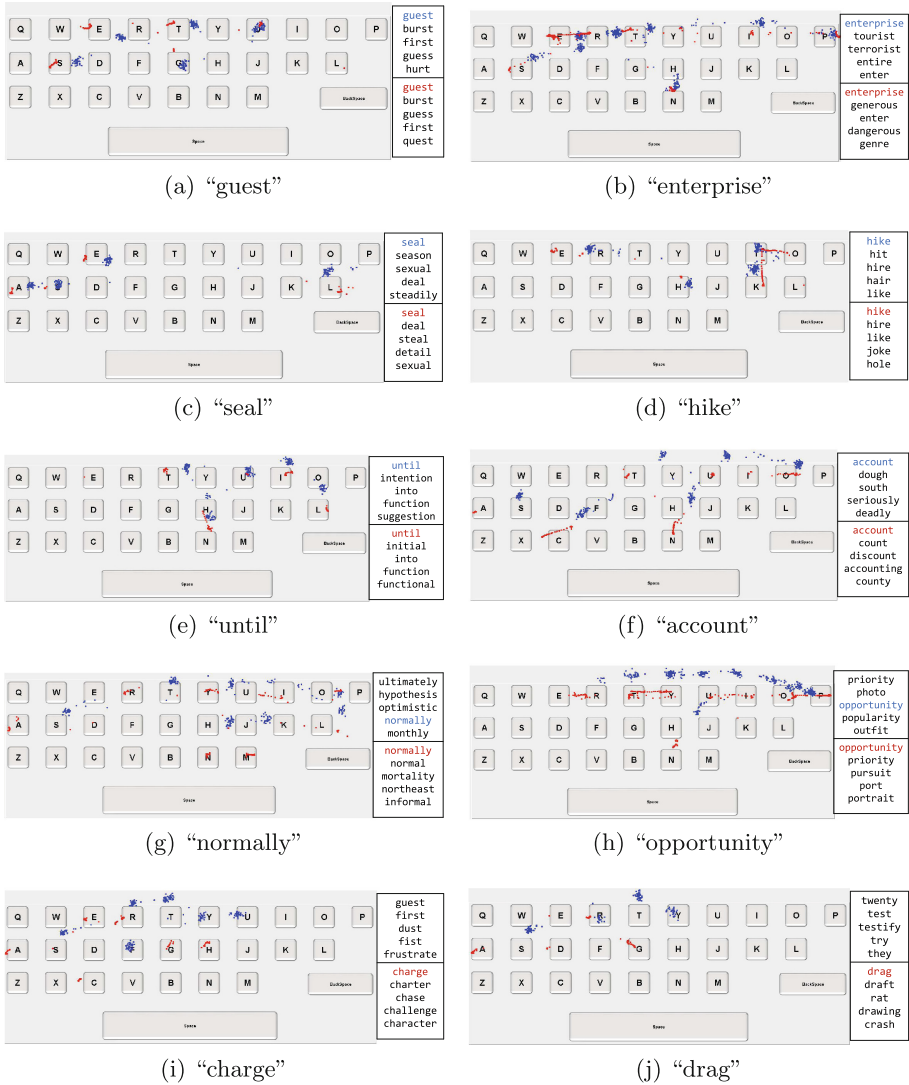
Fig. 9. Estimated gaze points of appearance-based method and eye tracker. They show the estimated points of typing ten words, “guest”, “enterprise”, “seal”, “hike”, “until”, “account”, “normally”, “opportunity”, “charge”, “drag”. The blue dots denote points estimated by the appearance-based method, and the red dots denote points by eye tracker. The upper right box shows top-5 words recommended using estimated points of the method, and the lower right box shows top-5 words using points of the eye tracker. (Color figure online)
