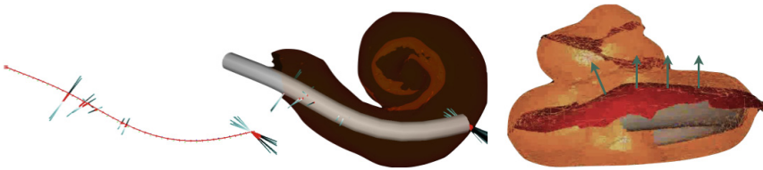
Fig. 3. (Left) The implant is modeled using beam elements and, (middle) its motion is constrained by contact and friction response to collision with cochlear walls. (right) Contact forces induces strain on the Basilar membrane.
