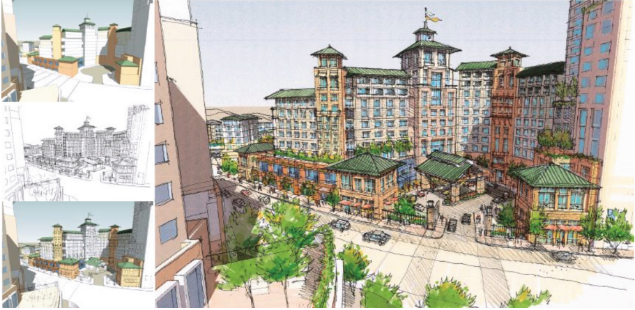
Fig. 2. 3D drawings for urban planning and industrial design. A process from professional practice for communicating solution concepts with a blend of computer and handcrafted renderings [44, 50]. New designs are often based off real object references, mockups or massing models for selecting viewpoints and rough shapes. These can be modeled manually in, e.g. , Google Sketchup (top-left), in some cases from reference imagery. The desired 2D views are rendered and manually traced into a reference curve sketch (center-left, bottom-left) easily modifiable to the designer’s vision. The stylized drawings to be presented to a client are often produced by manually tracing and painting over the reference sketch (right). Our system can be used to generate reference 3D curve drawings from video footage of the real site for urban planning, saving manual interaction, providing initial information such as rough dimensions, and aiding the selection of pose, editing and tracing. The condensed 3D curve drawings make room for the artist to overlay his concept and harness imagery as a clean reference, clear from details to be redesigned.
