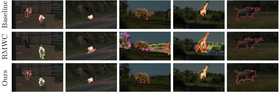
Fig. 7. Example results for object co-segmentation on the Safari dataset. Segmentation outputs are indicated as colored contours, where each color represents an instance. Compared to the state-of-the-art approach [34] (second row) and the baseline method [21] (first row) that often produce noisy segments, false positives or missing objects, our method obtains better segmentation results. Best viewed in color.
