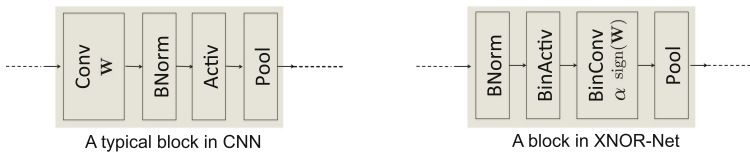
Fig. 3. This figure contrasts the block structure in our XNOR-Network (right) with a typical CNN (left).
