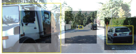
Fig. 1. In natural images, objects can appear at very different scales, as illustrated by the yellow bounding boxes. A single receptive field, such as that of the RPN [9] (shown in the shaded area), cannot match this variability.
