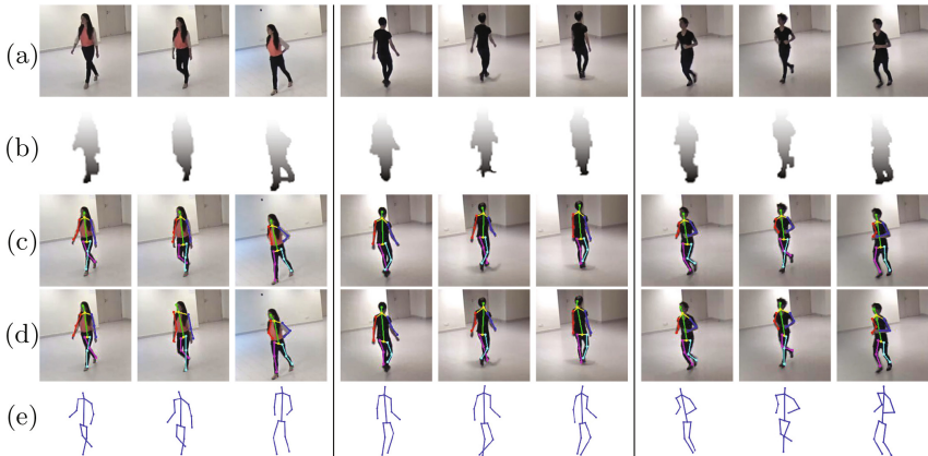
Fig. 8. Qualitative result of the proposed framework of 3 persons (left, middle and right) from the MCAD [41]. (a) Image sequence, (b) Computed height-maps, (c) Ground-truth of 2D joints, (d) Localized 2D joints, and (e) Recovered 3D motion.
